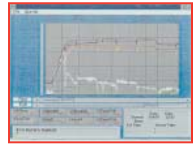
History Chart - historical charts with up to eight screen pens display data for each charge. The screen also has memo fields for annotation. Each screen may be printed as a report
